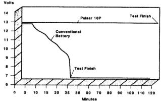
RESISTANCE TO VIBRATION is inherent to the Pulsar design. The test shown was completed at a very severe 10g 50hz rate that killed a conventional battery in a matter of minutes, while the Pulsar was unaffected after two hours. (Leaf hybrid)
