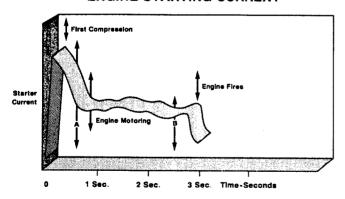
When a typical car is started, there is an initial in-rush current that starts the engine turning. This current then decreases to a constant cranking current, which continues until the engine fires. This whole process usually takes less than three seconds.
