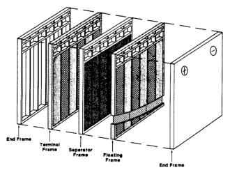
This is accomplished by a unique method of construction which involves the injection molding of four distinct types of frames, a terminal frame, floating frame, separator frame and end frame. In each of the active frames, expanded lead is molded into the plastic and, in turn, is pasted with active
