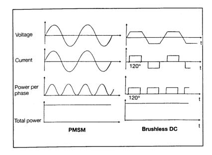
contains a large amount of harmonic current that produce motor heating, more noise, and a risk of torque pulsation that can affect gear tooth performance.
