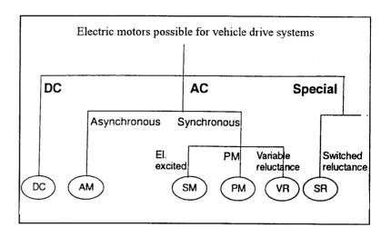
Each of these motors has its advantages and disadvantages. The major advantages with DC motors are that they are easy to control and the controllers are fairly inexpensive. The disadvantages are the commutation restrictions, the weight, and relative low efficiency.
