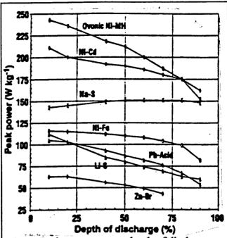
Fig 6. Peak power versus depth of discharge measured at Argonne for a number of EV battery types
