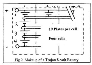
Each cell produces an electromotive force of 2.35 volts per cell. The Trojan 875 battery has four cells connected in series as shown by Fig 2. The combination produces a 9.4 volt battery open-circuit voltage at full charge.
