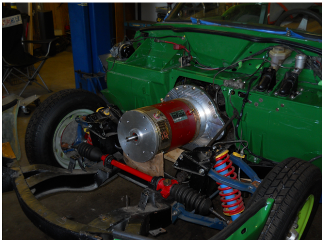
Bob's conversion showing motor mouting
