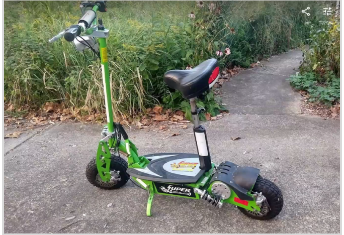
Ted's scooter he got from Bruce Lanzerotti and retrofitted it w two 18V Ryobi batteries
