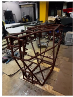
Primed frame after light sanding
