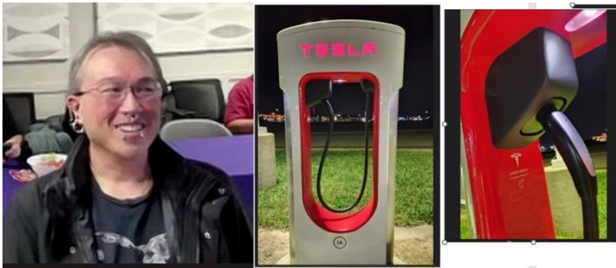
Ted Liu provided an in-depth analysis of the Tesla Supercharger with Magic Dock technology and how that allows vehicles with non-Tesla charging ports to charge at Superchargers.
